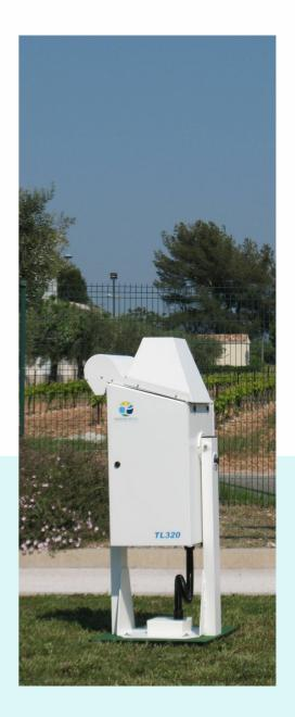
The ceilometer opto electronics are enclosed in a rugged housing protecting the sensor from extreme operating conditions. An automatic blower with heater ensures to keep the window clean and dry under all weather conditions.
